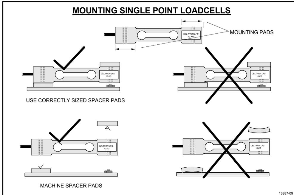
The spacer or pad that the loadcell is mounted to must lift the loadcell clear of the surrounding structure. Usually 5mm would be the minimum spacer thickness. The spacer or pad **must be flat, preferably machined**. If the pad is not flat, the loadcell will be distorted when it is bolted up.
