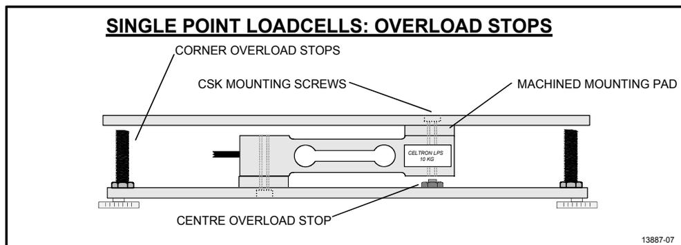
Overload stops must be at least 10mm diameter. They should preferably be a fine thread and **MUST** have a machined flat face on the overload stop. Some loadcells (Celtron MOC and HOC) come complete with tapped recesses specifically for overload stops.
